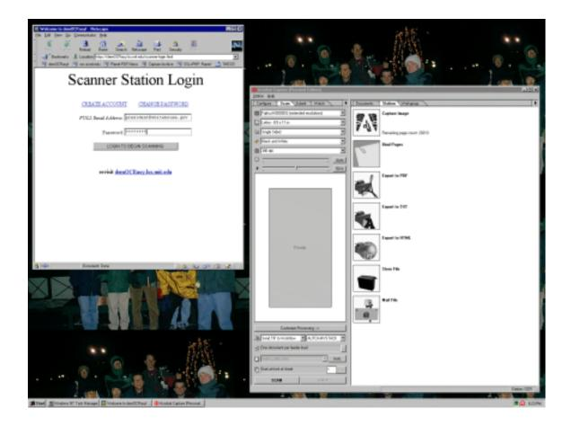
On the top-left you see the SSL-enabled Netscape login-box which we use to guide the user through their scanning session. On the bottom-right you see Adobe Capture 3.0, which controls the scanner and performs the OCR. The per-document "SCAN" button is in Capture's lower left-hand corner: this is the *only* button users will need to touch while logged in.
